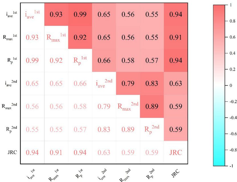
Figure 6: First- and second-order morphological parameters and JRC correlation heatmap.
