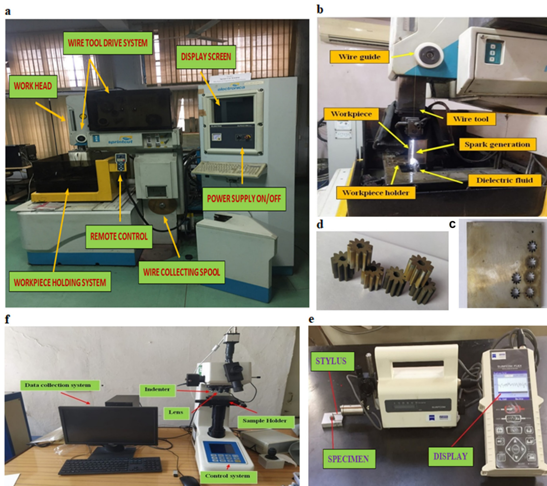
Figure 3: Pictorial view of process flow chart: (a) WEDM machine setup, (b) processing of superalloy 690 by WEDM, (c and d) miniature spur gears and their cavity in the plate after WEDM, (e) SR measurement, and (f) microhardness analysis.
