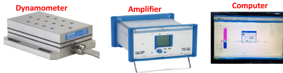
Figure 2: Cutting force measuring setup.
