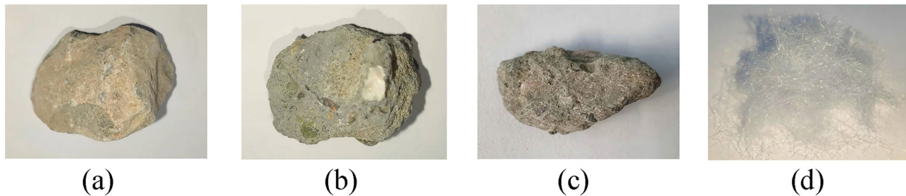
Figure 1: Appearance of coarse aggregate and PPF: (a) NCA, (b) RCA, (c) RCA-20, and (d) PPF.
