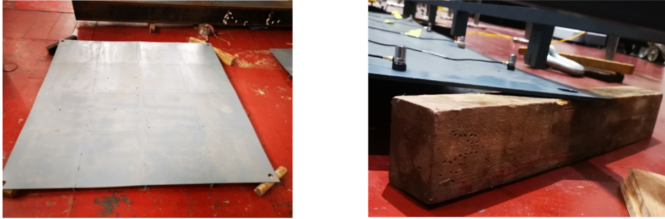
Figure 5: Simulation of simple boundary conditions.
