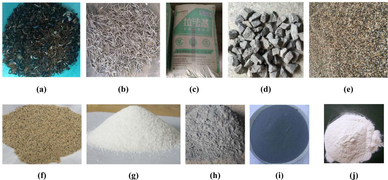
Figure 1: Composition of RSF-reinforced concrete. (a) RSF. (b) PSF. (c) Cement. (d) Crushed stone. (e) Bean stone (f). Natural sand. (g) Quartz sand. (h) Fly ash. (i) Silica fume. (j) Superplasticizer.
