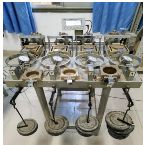
Figure 8: Quadruple constant strain direct shear apparatus.
