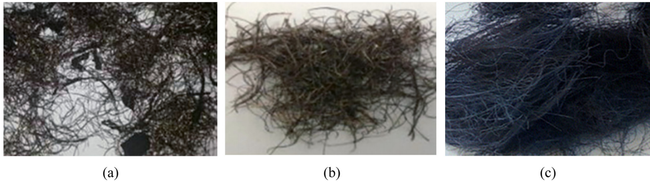
Figure 1: WTSFs obtained using different recycling techniques [29]. (a) Shredding technique, (b) cryogenic technique, and (c) pyrolysis technique.
