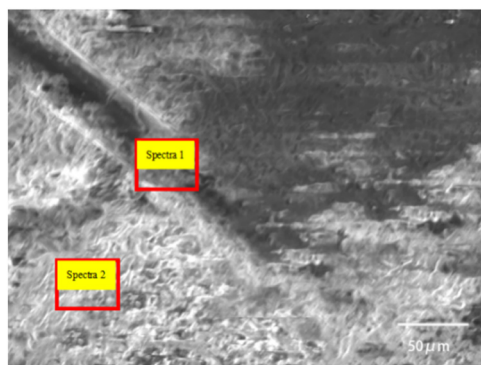
Figure 8: The location of the groove left by pullout fiber and mortar in B_1 specimen.
