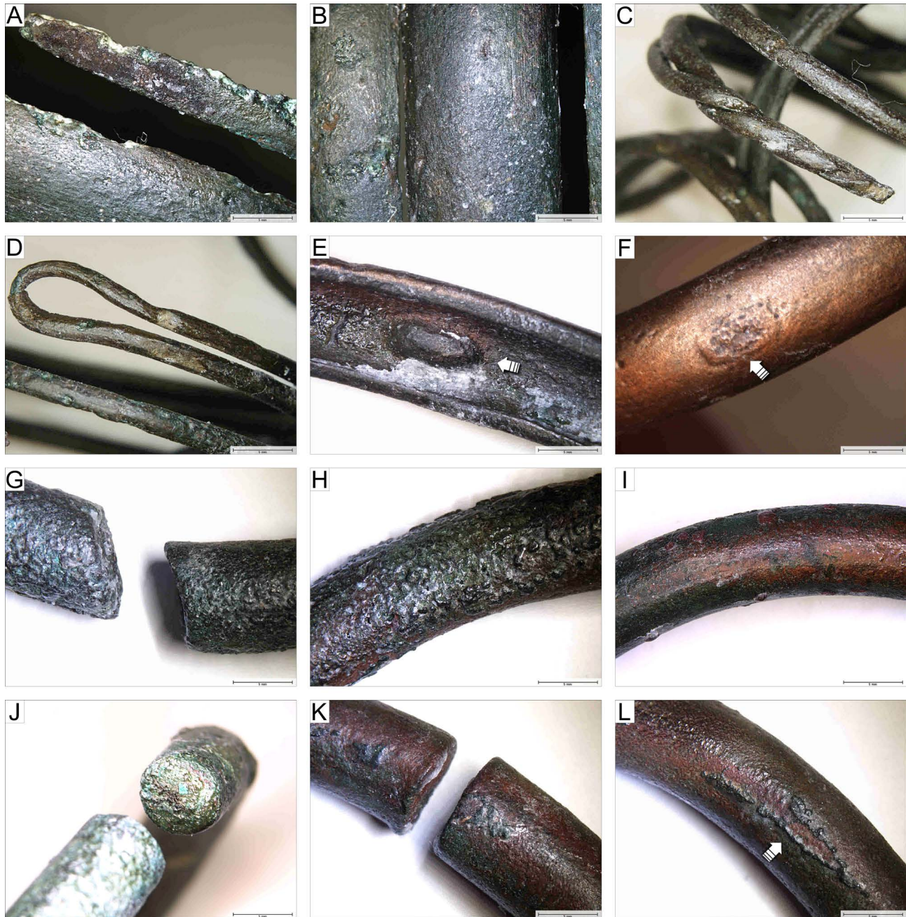
Fig. 7: Photomicrographs of the artefacts showing the macrostructures typical of casting and plastic forming. A–B – spiral bracelet EI-1; C–D – wire coils EI-5; E–F – bracelet EI-7; G–H – solid bracelet EI-8; I–J – solid bracelet EI-9; K–L – solid bracelet EI-10 (photographs: P. Jurecki). See text for further details.
