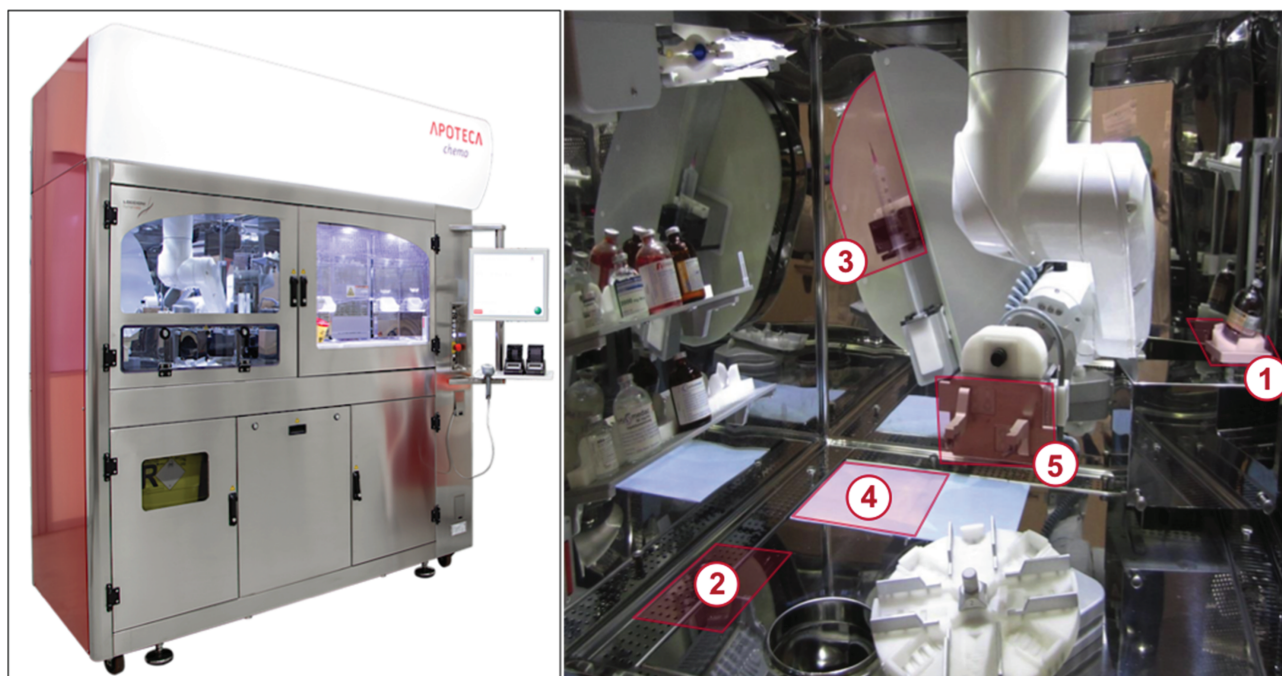
Figure 2: Robotic system APOTECACHemo, Loccioni Group, Italy, (left side in total); working area (right side) with marked sampling sites: (1) balance, (2) surface beneath the shelves, (3) dosing device, (4) surface beneath the dosing device, (5) gripper of the robotic arm.
