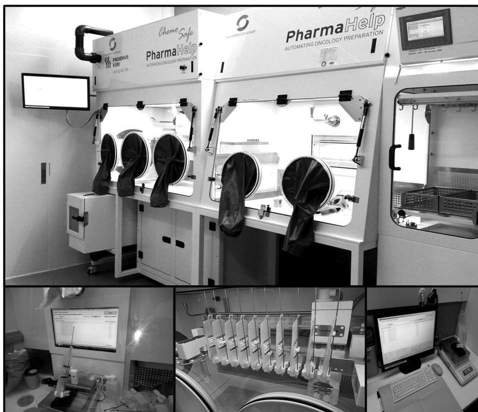
Figure 1: PharmaHelp ® automated compounder: pre-process, production and post-process zone (from the left to the right on the photo).
