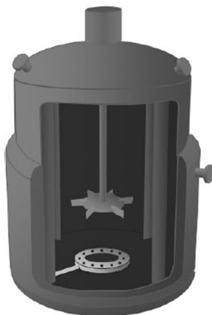
Figure 3: Schematic of a stirred tank reactor with Rushton turbine and gas sparger.
