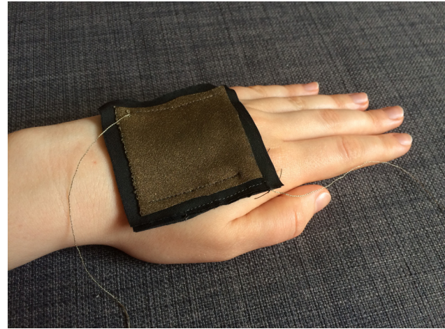
Figure 3: A photograph of the prototype fabric-based tactile sensor for a robot companion that was shown to participants. Participants were told that several such sensors could be placed across the robot’s body, and that they could be used to detect the intensity and/or type of touch being enacted on the sensor. Participants were asked to give feedback and share any concerns they might have with such a design.
