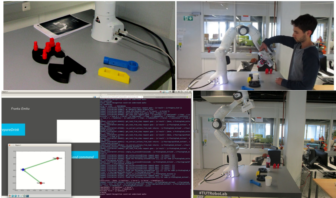
Figure 7: Top Left: Cranfield benchmark parts. Bottom left: Generated action plan (graph) and graphical user interface. Top right: demonstration of skills for human-robot collaboration. Bottom right: Robot independent execution of a task.
