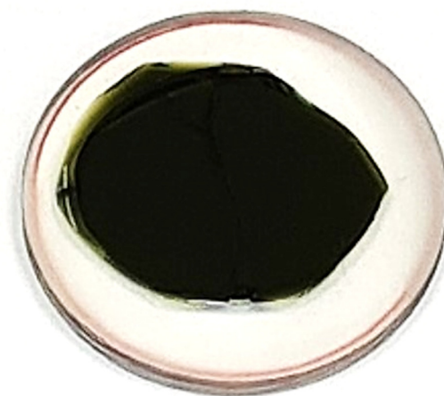
Figure 1: Physical appearance of the synthesized Copper(II) oxide reinforced glass sample BCV0.5.
