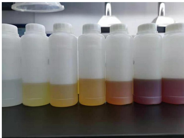
Figure 2: Ageing insulating oil colour change.
