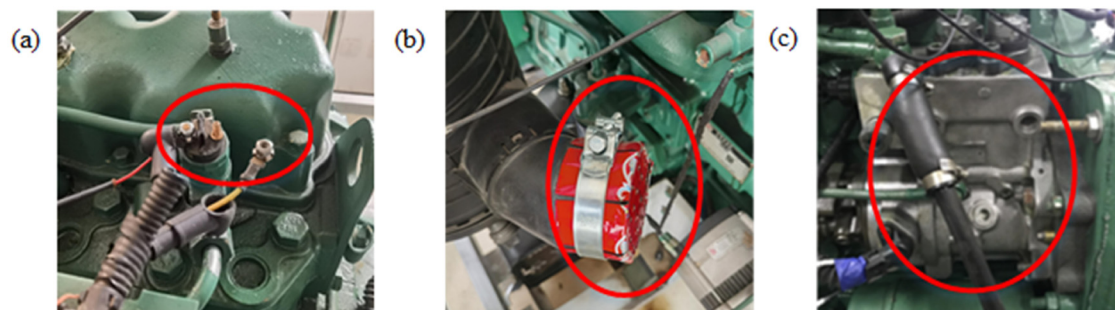
Figure 9: (a) Disconnect the startup power cord; (b) install the metal cover; and (c) replace the defective fuel injection pump.
