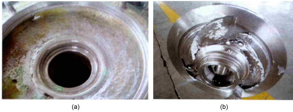
Figure 6: Failure of the shield pump [20]: (a) flow passage component and (b) impeller maintenance status.
