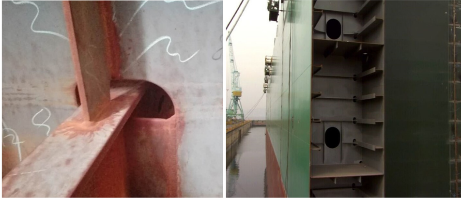
Figure 1: Cutouts and slots form on the ship constructions.
