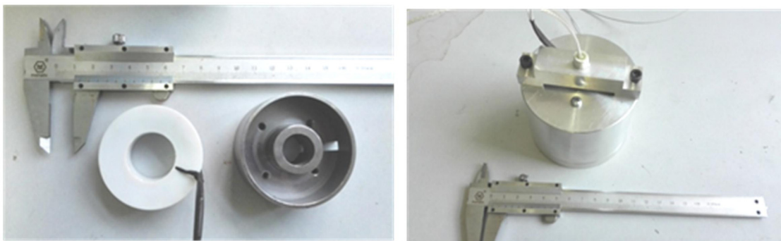
Figure 10: Parts and assembled parts of the magnetic suspension stabilizer.
