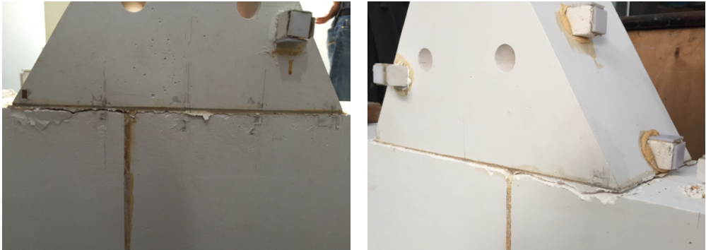
Figure 16: Failure pattern of dam (left and right sides of the model)
