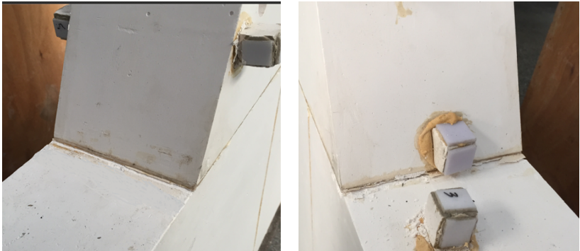
Figure 17: Local failure pattern of dam body (dam heel and foundation)
