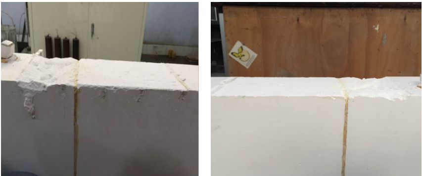
Figure 19: Failure pattern of foundation plane (left and right sides of the model)
