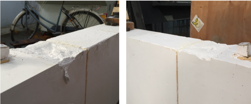
Figure 18: Failure pattern of foundation plane of dam body (toe of dam and foundation)
