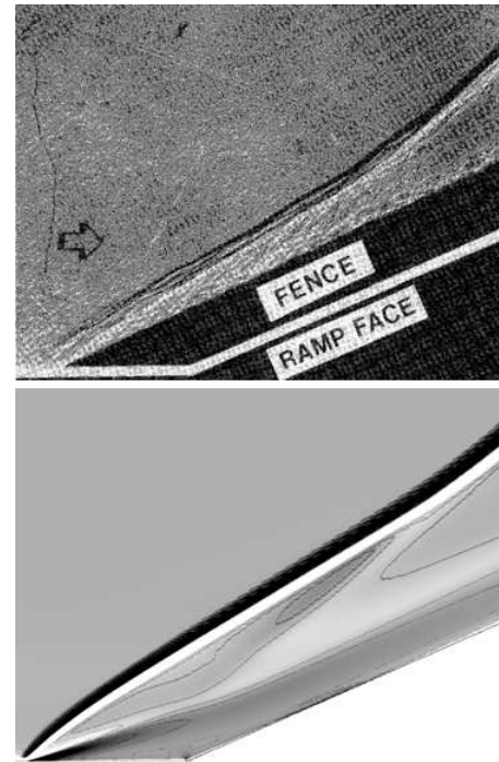
Figure 2: Comparison between the experimental [25] (upper) and numerical (lower) shadowgraphs
