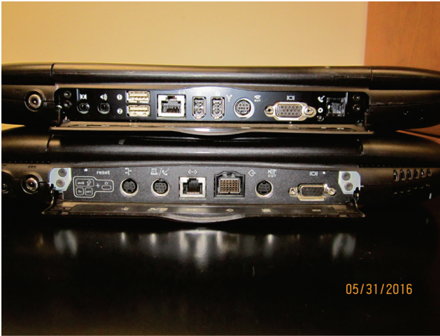
Figure 2: Rear connections for Apple Powerbook G3 (“Wallstreet,” 1998) on the bottom; Apple PowerBook G3 (“Pismo,” 1999) on the top.
