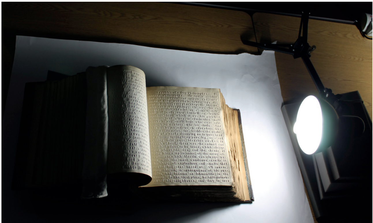
Figure 8: Example of Lighting Setup to Bring out Surface Relief of Embossed Books. The lamp is placed on only one side (uneven) with light directly across the page at an oblique angle approaching 180 degrees (raking light), 2015, Perkins School for the Blind Archive.
