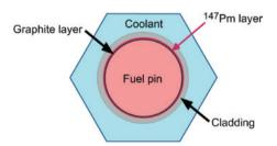
Fig. 4.61.1: The beta-ray backscatter technique requires a layer of 147Pm between the cladding and the graphite layer to measure the thickness of the graphite along the inner surface of the cladding tube. (Modified from [308]).
