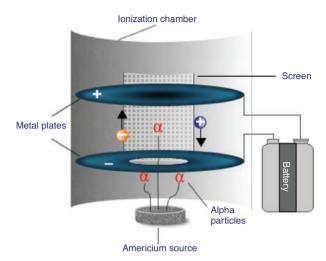
Fig. 4.95.1: In a smoke-free chamber, the ionized air molecules create a current between the two metal plates having a voltage difference. Current flows continuously until smoke disrupts the current, at which time the alarm sounds. (Diagram Source: US Environmental Protection Agency) [615].
