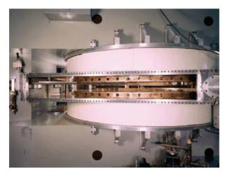
Fig. 4.44.2: The 88-Inch cyclotron was used to produce both light and heavy ions, including 94Ru and 95Ru. (Photo Source: Lawrence Berkeley National Laboratory) [336].
