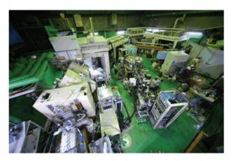
Fig. 4.113.2: GARIS (Gas filled recoil ion separator) used to synthesize nihonium (kindly provided by RIKEN).
