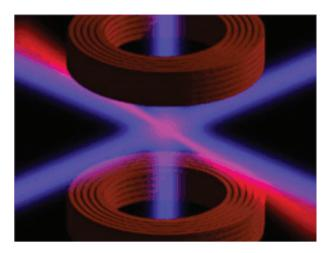
Fig. 4.70.2: The insides of the National Institute of Standards and Technology's (NIST) optical atomic clock. The red rings are magnetic coils and the red laser beam is an optical lattice. The intersecting violet lasers cool the ytterbium atoms. (Image Source: National Institute of Standards and Technology, 2006) [497].
