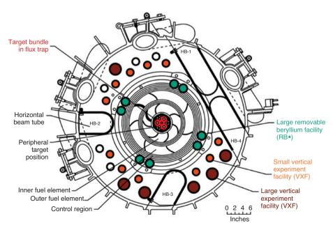
Fig. 4.96.1: Schematic drawing of the inside of a reactor core at the Oak Ridge National Laboratory's High Flux Isotope Reactor facility. 244Cm is used as the target in the flux trap. (Image Source: Oak Ridge National Laboratory) [619].
