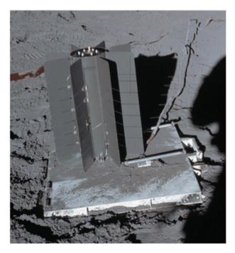
Fig. 4.94.1: <sup>238</sup>Pu is used in the SNAP-27 radiothermal generator as a heat source to produce electricity to power spacecrafts, such as for Apollo missions 12, 14, 15, 16, and 17. (Image Source: NASA) [612].
