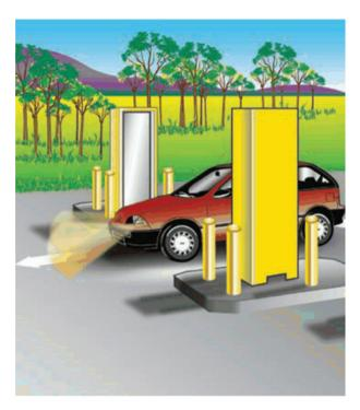
Fig. 4.2.1: Radiation detectors are installed in many areas to screen people, vehicles, and cargo for radioactive materials. <sup>3</sup>He detectors are sensitive to thermal neutrons and are used to detect isotopes of uranium and plutonium that might be used in nuclear weapons, along with other sources that produce neutrons by radioactive decay. (Image Source: U.S. Government Accountability Office) [33].
