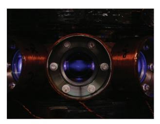
Fig. 4.66.1: Magneto-Optical Trapping (MOT) of isotopes of dysprosium. (Used with permission from: Prof. Benjamin Lev, Stanford University) [466].
