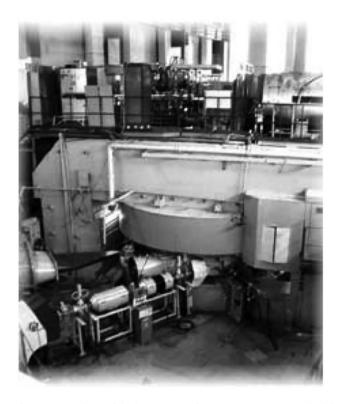
Fig. 4.116.1: Photo of the heavy ion cyclotron U-400 at JINR in which livermorium was synthesized. (Photo Source: Lawrence Livermore National Laboratory) [675].
