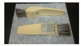
Fig. 4.84.1: Staticmaster<sup>TM</sup> Alpha lonizing Brushes for cleaning optical surfaces and photographic films have a soft, nonabrasive brush and a 210Po cartridge. (Photo Source: Reston Stable Isotope Laboratory of the U.S. Geological Survey) [564].
