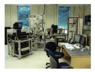
Fig. 4.18.2: The U.S. Geological Survey 40Ar/39Ar geochronology laboratory in Denver, Colorado uses a custom-built argon extraction line connected to a Mass Analyzer Products (MAP) 215-50 mass spectrometer with a differentially pumped dual laser setup. (U.S. Geological Survey 40Ar/39Ar Geochronology Laboratory) [175].
