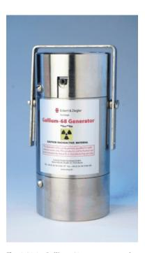
Fig. 4.31.1: Gallium-68 generator used to provide medical therapy with the positron-emitting radionuclide 68Ga. The parent radionuclide, 68Ge, has a half-life of 271 days and has been used as the source of 68Ga, which has a half-life of only 68 min. Image kindly provided by Dr. Anatolii Razbash, Cyclotron Co. Ltd., Obninsk, Russia.
