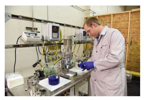
Fig. 4.89.1: The Medical Actinium for Therapeutic Treatment (MATT) is a separations process that recovers <sup>225</sup>Ac from unused nuclear fuel so the isotope can be used in cancer treatment and research. (Image Source: Idaho National Laboratory) [588].
