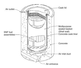
Fig. 4.92.2: DUCRETE cask diagram. DUCRETE is being proposed as a suitable material for the storage of radioactive waste. (Diagram Source: Argonne National Laboratory) [601].
