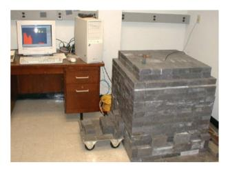
Fig. 4.63.2: <sup>152</sup>Eu is used as a reference source for calibrating gamma-ray spectrometer systems like the one pictured here. (Photo Source: Snyder and Duval, 2003. U.S. Geological Survey Open-File Report 03-029) [450].
