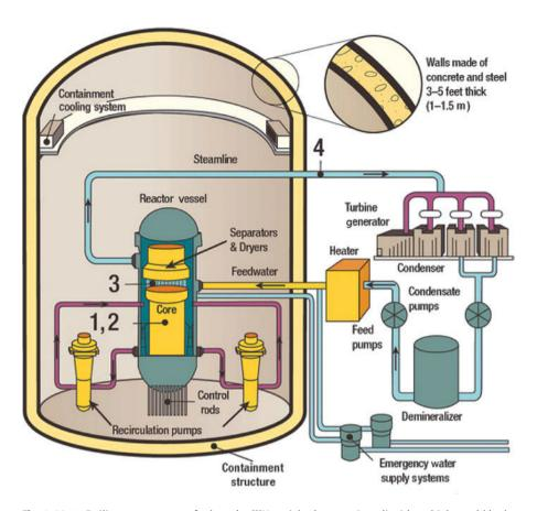
Fig. 4.92.1: Boiling water reactor fuel can be 235U enriched as uranium dioxide, which would be located in the core and is identified as "Core". (Diagram Source: U.S. Nuclear Regulatory Commission) [602].
