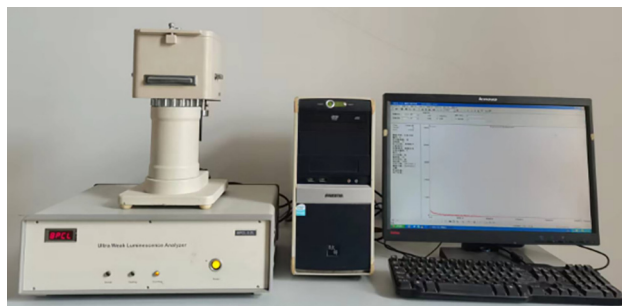
Figure 1: The BPCL-ZL-TGC ultra-weak photon acquisition instrument (taken by the author using a mobile phone in the school's food processing laboratory, permission and authorization have been obtained from the laboratory).
