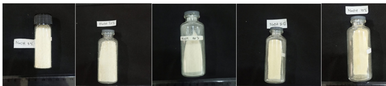
Figure 2: The appearance of produced Na-CMC from nata de pina under various NaOH concentrations.
