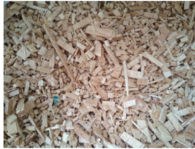
Figure 2: Particle from veneer waste.
