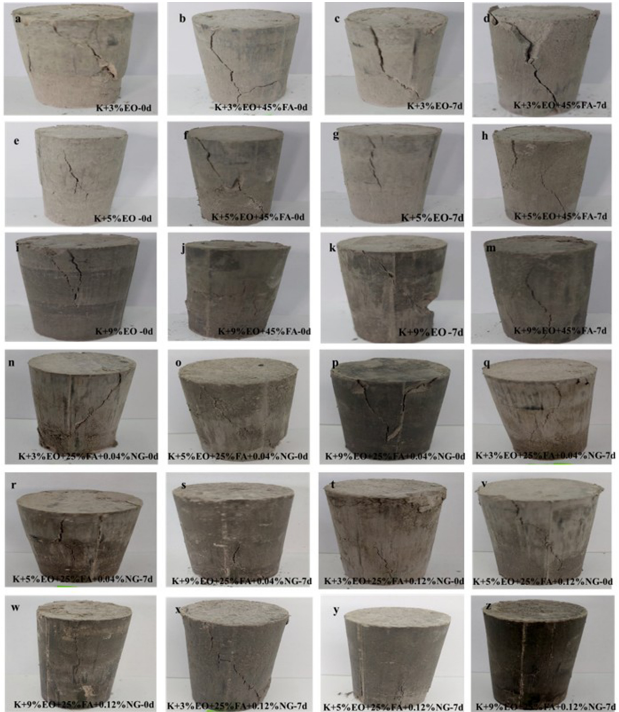
Figure 14: Fracture modes of the samples for 0 and 7 days curing period.
