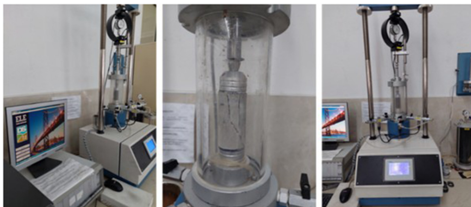
Figure 6: Unconfined compression strength (UCS) testing performed using a triaxial apparatus.
