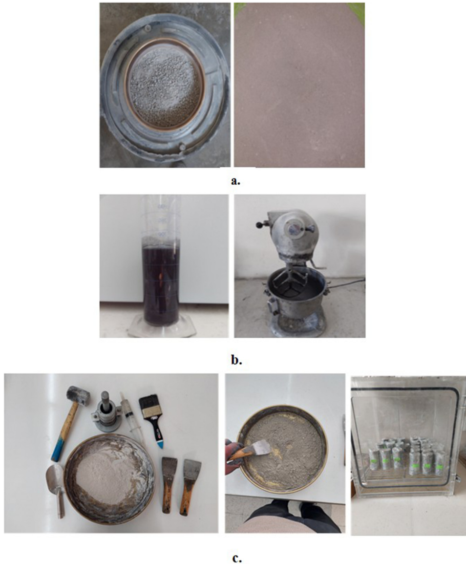
Figure 5: Preparation of the soil samples. (a) the kaolin-waste engine oil mixture, (b) nanographene solution, and (c) contamination process and test specimens.
