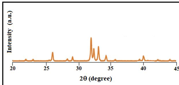
Figure 2: XRD analysis of pure HA synthesized using CMFS.
