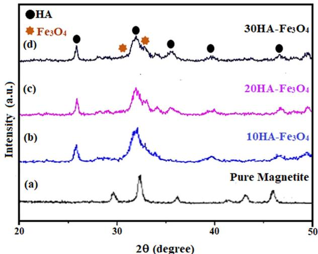
Figure 3: XRD pattern of HA-Fe<sub>3</sub>O<sub>4</sub> nanocomposites: (a) Pure magnetite, (b) 10HA-Fe<sub>3</sub>O<sub>4</sub>, (c) 20HA-Fe<sub>3</sub>O<sub>4</sub>, and (d) 30HA-Fe<sub>3</sub>O<sub>4</sub>, prepared at pH 11 in 5 min in CMFS.
