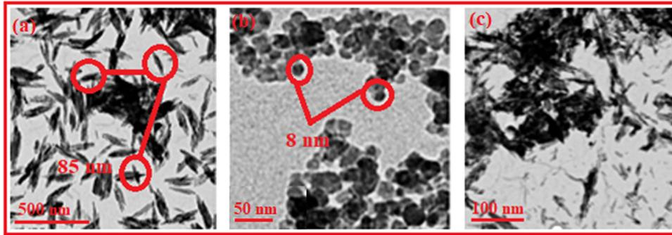
**Figure 4:** TEM images of (a) pure HA, (b) pure magnetite, and (c) HA-Fe<sub>3</sub>O<sub>4</sub> nanocomposites.
