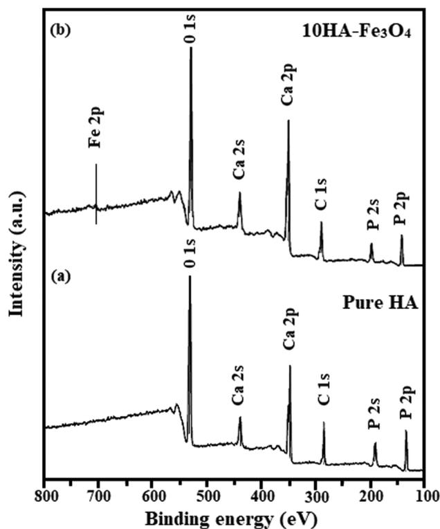
**Figure 5:** The XPS survey spectrum of (a) Pure HA and (b) 10HA-Fe<sub>3</sub>O<sub>4</sub> nanocomposite.
