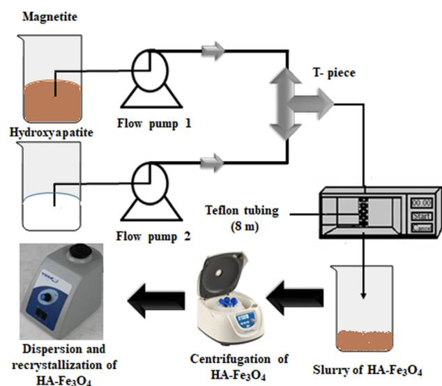
Figure 1: Schematic diagram for the preparation of HA-Fe<sub>3</sub>O<sub>4</sub>.
