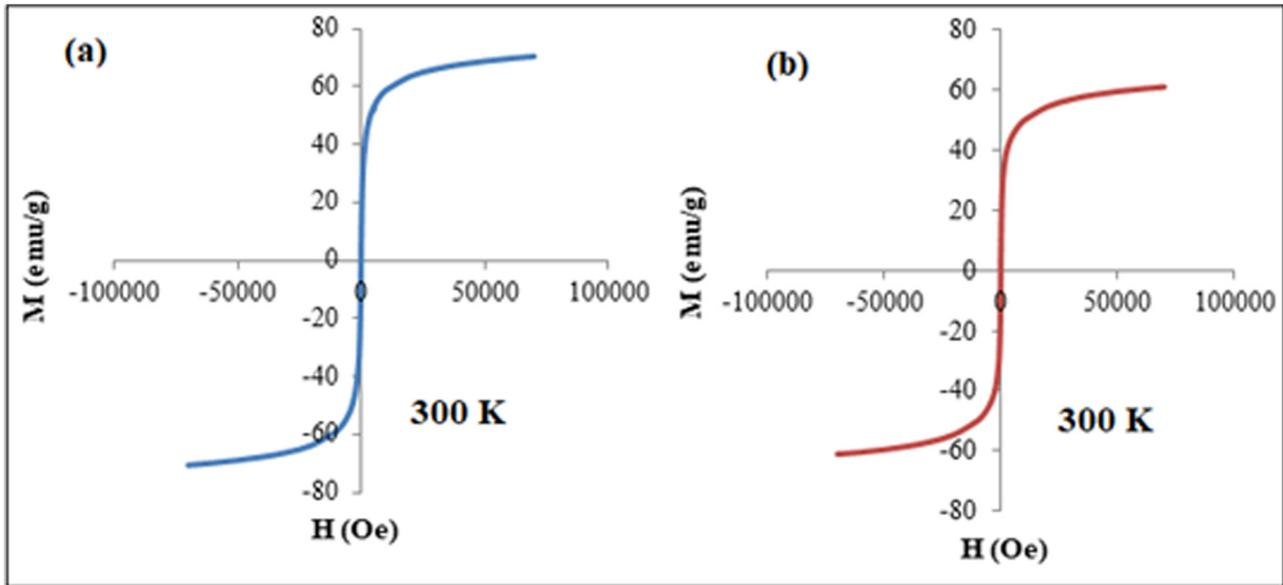
**Figure 6:** The saturation magnetization values  $M_s$  of (a) pure Fe<sub>3</sub>O<sub>4</sub> nanoparticles and (b) 30HA-Fe<sub>3</sub>O<sub>4</sub> nanocomposites, respectively, at 300 K.
