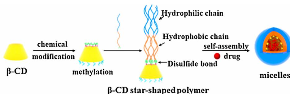
**Figure 8:** Detailed synthetic routes of a series of CD-block copolymers complex. Adopted from Li *et al.* [88].
