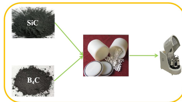
Figure 2: Procedure of ball milling.
