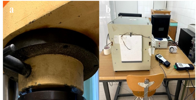
Figure 2: Flexural test (a) and insulating cube employed to measure thermal properties (b).
