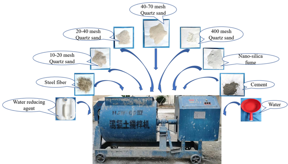
Figure 3: Composition of UHPNC and mixing device.
