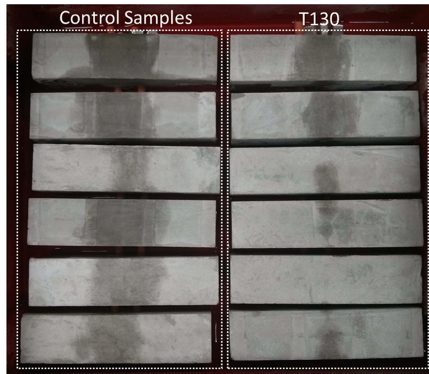
Figure 13: Sorptivity measurements are taken over a 28-day healing period. Comparison of later absorbed by cement (left) control cement paste samples and (right) cement paste samples containing 4% T130 microcapsules (polyurea microcapsules). Testing is after a 7-day healing period [94].
