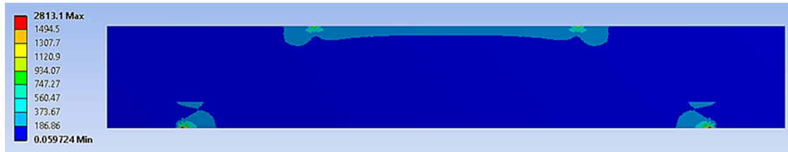
Figure 3: The example of the von Mises stress distribution for the geometrical sandwich panel using a four-point bending simulation under 70% of cyclic loading conditions.
