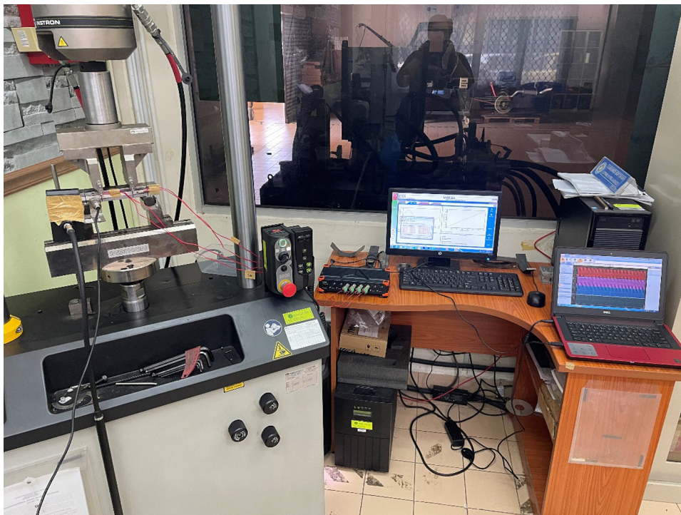
Figure 8: The set-up of the four-point bending test using Fatigue Servo Hydraulic Machine and a Dewesoft Data Acquisition system.
