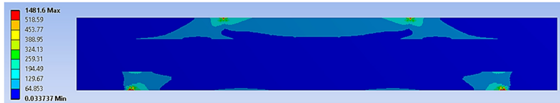
Figure 4: The example of the shear stress distribution for the geometrical sandwich panel using a four-point bending simulation under 70% of cyclic loading conditions.
