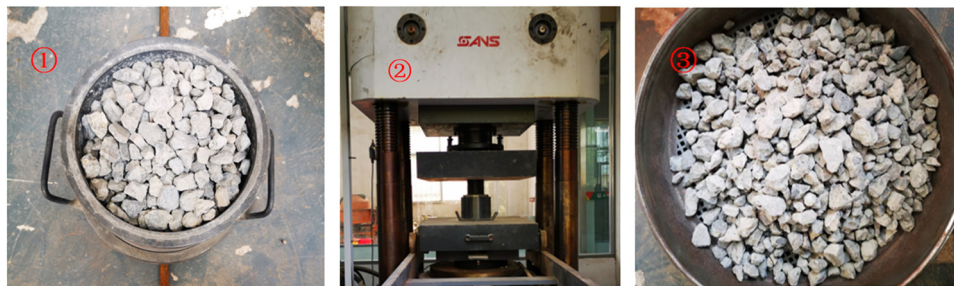
Figure 4: Determination process of crushing value of RA. (1) Sample and put into the mold; (2) Apply load; (3) Sieve the sample.
