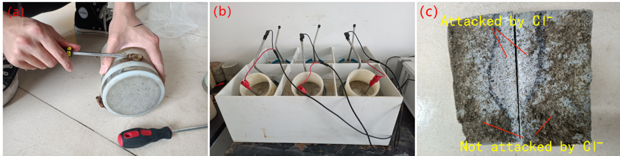
Figure 7: RCM test procedure of GOPARMs: (a) rubber sleeve installation; (b) power penetration; (c) section color change after spraying silver nitrate.
