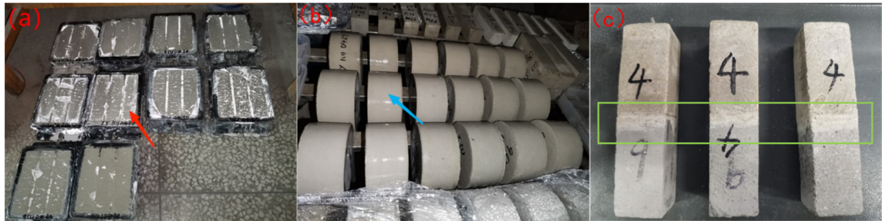
Figure 2: Photos of GOPARMs specimens: (a) compressive and flexural strength test (red arrow-prism); (b) resistance to chloride ion permeability test (blue arrow-cylinder); (c) bending bond test (green rectangular-new/old interface).
