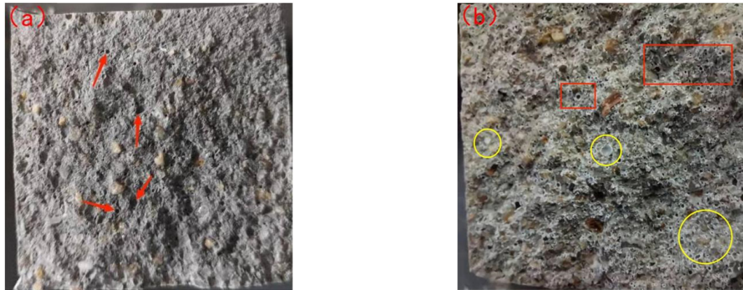
Figure 4: Classic section morphology of GOPARMs: (a) P0G0 group (red arrows—pores); (b) P5G3 group (yellow circles: polymer films and; red rectangles: air bubbles).
