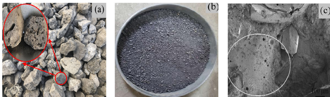
Figure 1: The appearance of SS: (a) SS stone; (b) SS sand; and (c) internal appearance.
