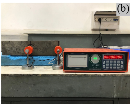
Figure 3: (a) Freezing-thawing specimens and (b) measurement of relative dynamic elastic modulus.
