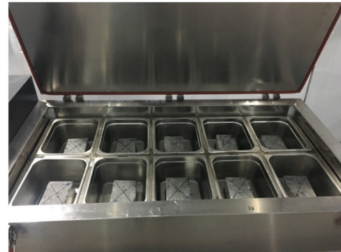
Figure 6: Instrument used for frost resistance test.
