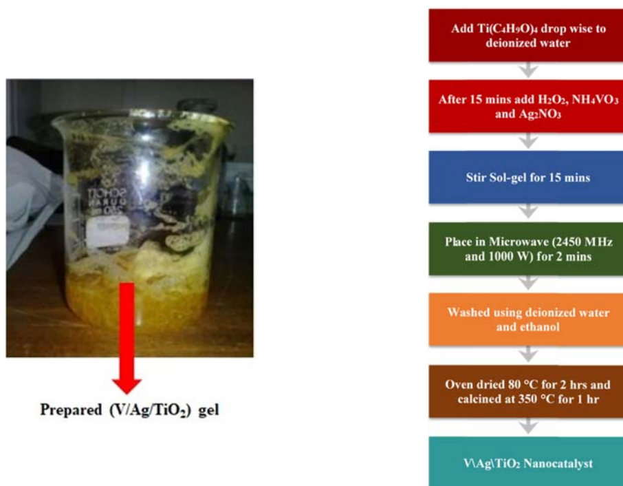
Figure 1: The schematic illustrations and sample preparation for the fabrication procedure.
