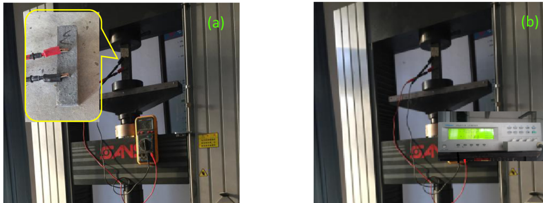
Figure 2: The piezoresistive test configuration of MNTSM or MNT/CM with two-electrode method: (a) DC resistance (yellow box – MNTSM or MNT/CM specimen with two electrodes); (b) AC impedance.
