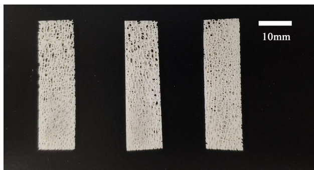
Figure 1: The configuration of the bone slice after degreasing.
