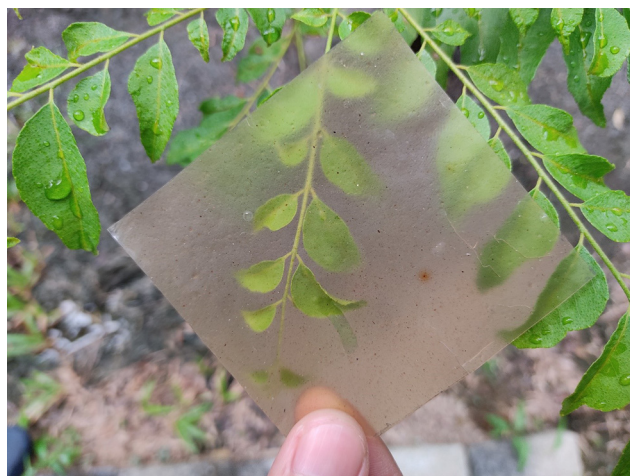
Figure 1: Transparent film of CEO-reinforced SPN/SPS biocomposite film.
