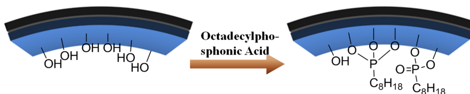
Figure 5: Selective modification of the inner surface by octadecylphosphonic acid proposed by Lvov et al. [19]
