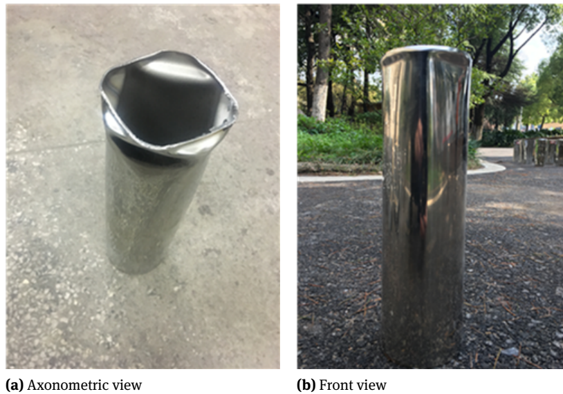
Figure 9: Failure mode of hollow stainless steel tube
