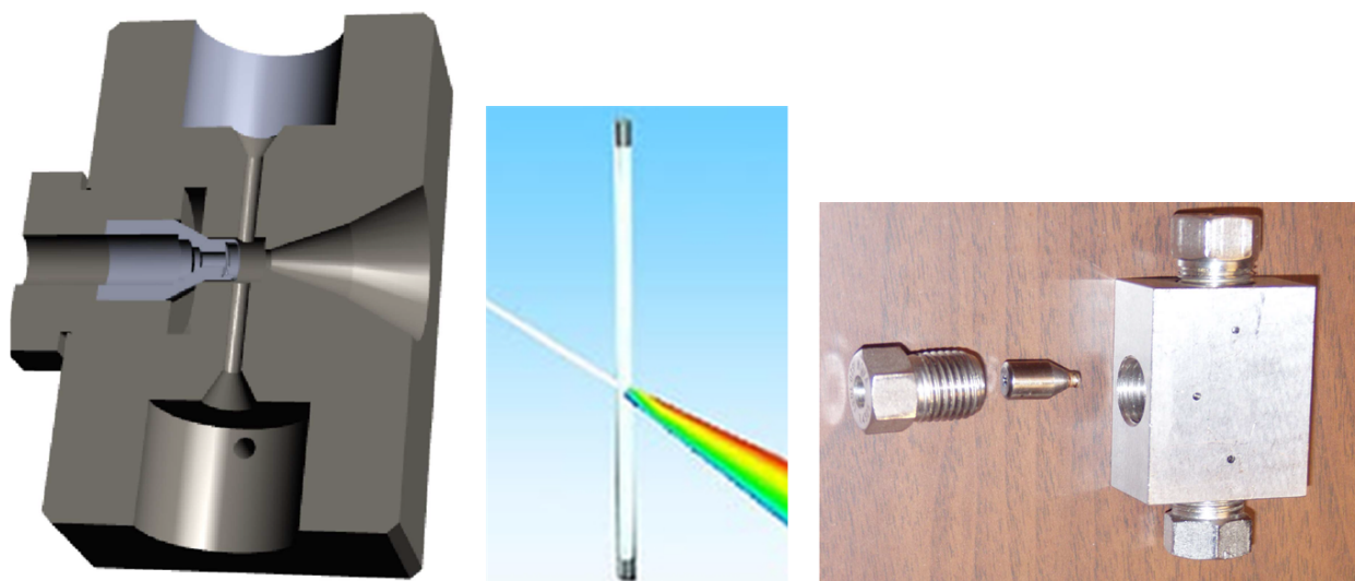
Figure 7: Horizontal cut through the hydrostatic high pressure cell (left) and the flexible polymer capillary (diameter 1.5 mm) containing the sample which fits into the central channel of the cell (middle). The beam passes from the left (entrance window) to the right (exit-window). The picture to the right shows the actual cell used at the SAXS-beamline at ELETTRA with the entrance window detached. On the right and left sides of the cell the high-pressure tubings for the pressure transmitting fluid (water) can be connected
