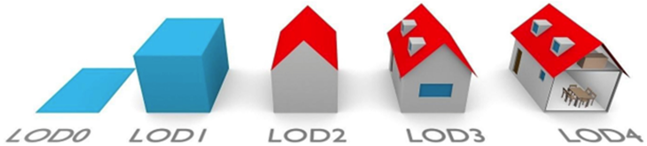
Figure 3: The five LODs of CityGML 2.0 From “An improved LOD specification for 3D building models,” by Biljecki et al. [73].
