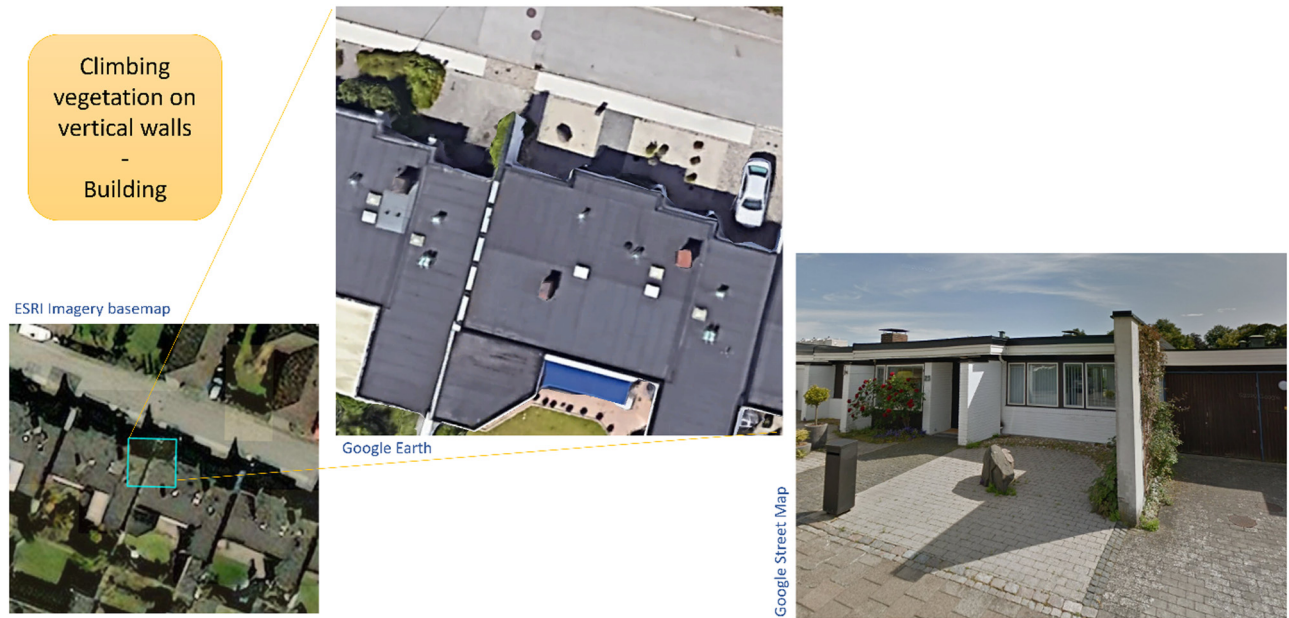
Figure A5: Screenshots over Vändåkersvägen 21, Malmö, Sweden showing how a NMD raster cell (left photo) has wrongfully been classified as forest , when it is a building façade with climbing plants.
