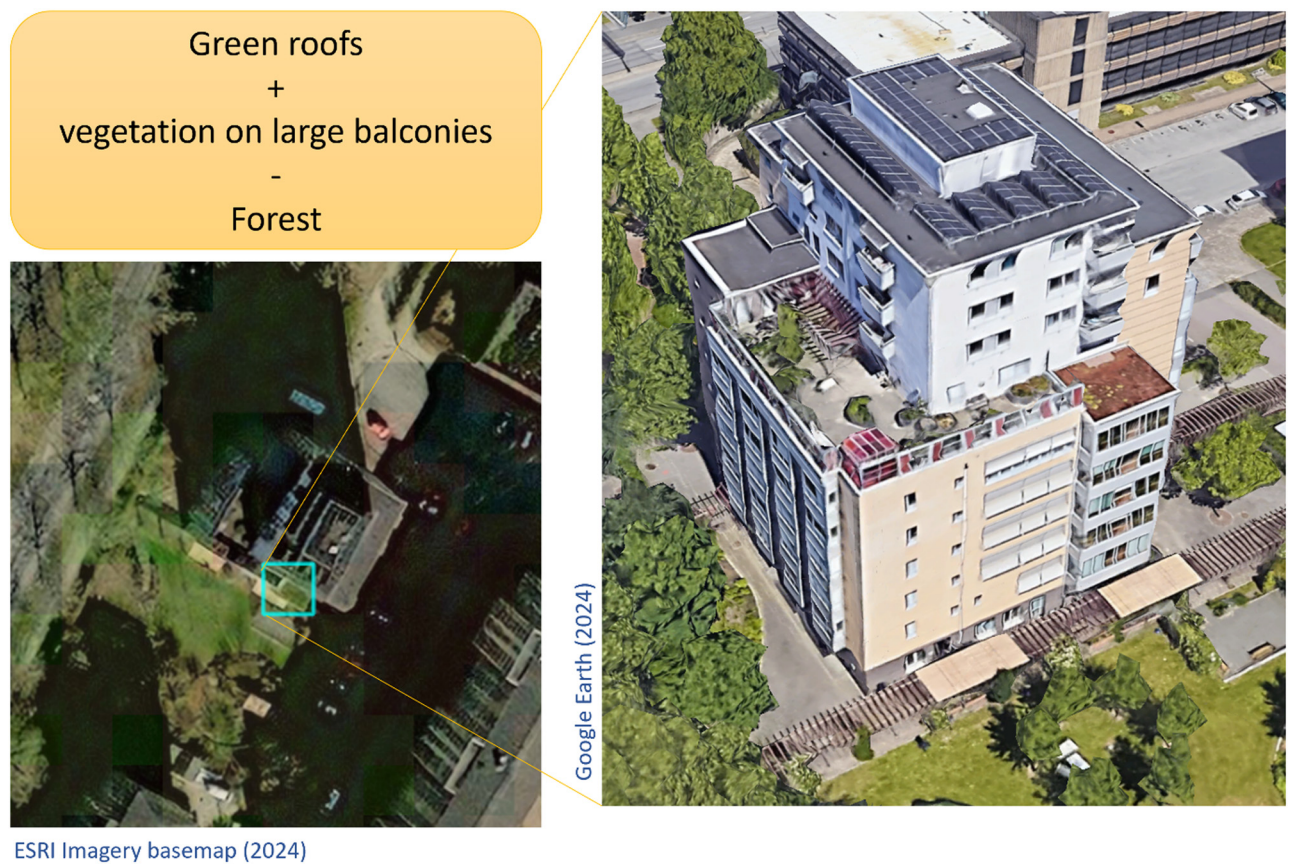
Figure A2: Screenshots over Stensjögatan 66, 217 65 Malmö, Sweden showing how a NMD raster cell (left photo) has wrongfully been classified as forest, when it is a building.
