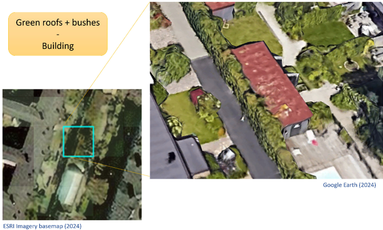
Figure A3: Screenshots over Vilebovägen 25, 217 63 Malmö, Sweden showing how a NMD raster cell (left photo) has wrongfully been classified as forest , when it is a building with a green roof.
