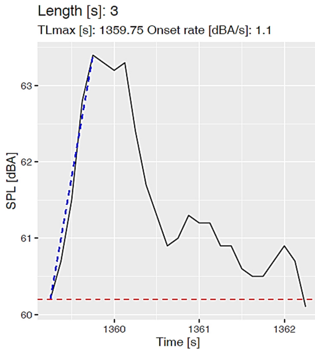
Figure 9: Example of the A-weighted SPL time history of a detected event. The horizontal red dotted line corresponds to the threshold for the event detection L_p and the inclined blue line connects the SPL at the start time with the maximum SPL of the event.
